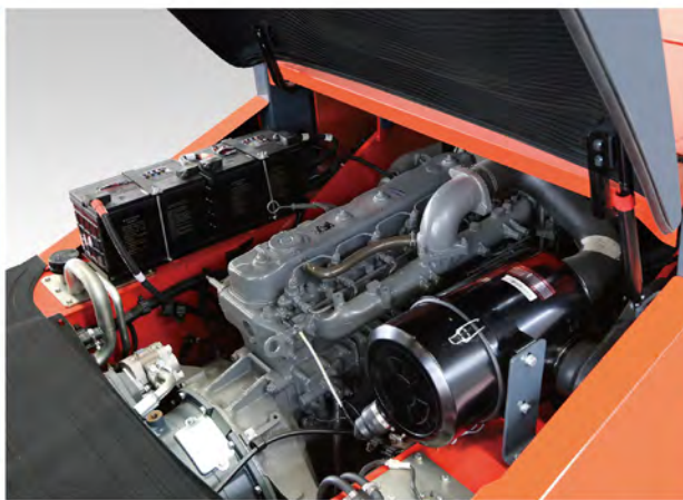
Standard 9 inch air filter with iron shell is helpful to extend maintenance period.
