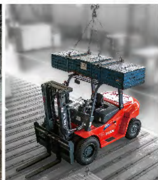
Impact test of overhead guard
