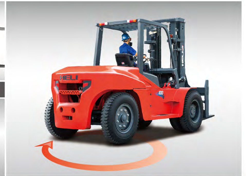
Large steering angle axle is equipped to get smaller turning radius.
